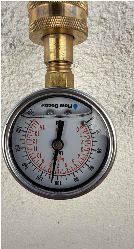
A. Plumbing Supply, Distribution Systems, and Fixtures: Static Water Pressure Reading Over 80 psi
